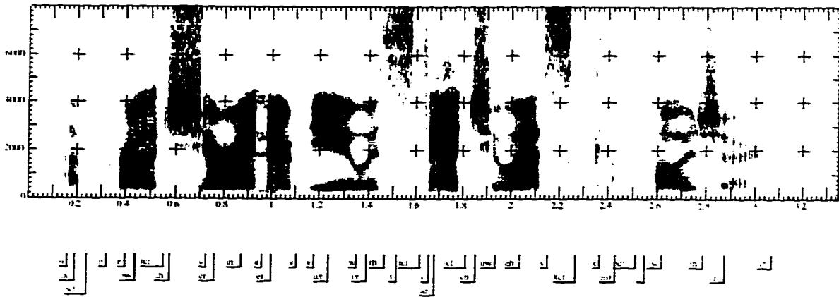
Figure 7.11: Spectrogram of the utterance “Approach your interview with statuesque composure” spoken by a female speaker. The alveolar /s/ fricatives at about 1.5 and 2.1 seconds have strong energy starting at about 4000 Hz, whereas the palatal affricates at 0.55 and 1.82 seconds and the palatal fricative /ʒ/ at 2.77 seconds have strong energy starting at about 2000 Hz and 2300 Hz, respectively.
